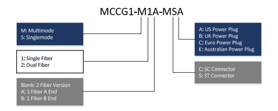
1. Transmission distance is limited by optical loss of the fiber and loss introduced by connectors, splices and patch panels. Fiber bandwidth also limits the transmission distance. 2. Please select the power plug from US Standard, Euro 2 Circular, UK 3 Pin square or Australian Standard when placing order.
